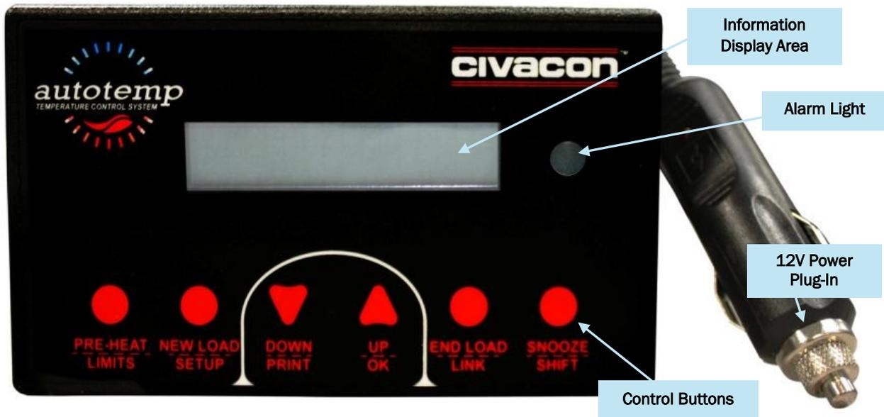
*Figure 2. In-Cab Display Unit, Part No. 3601T*
