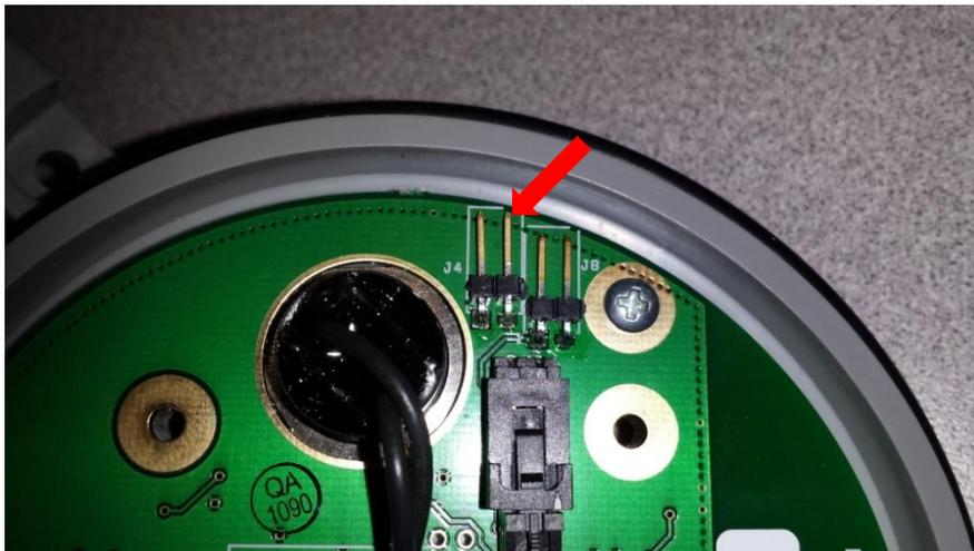
**Figure 11. Valve Disable Jumper Placement (J4)**
